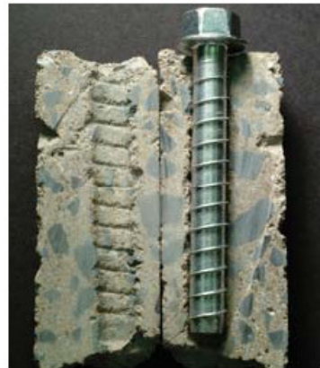
This core shows how the Titen HD undercuts the base material
