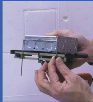
Adjust the electrical box cutting blade on the QC Hot Knife
